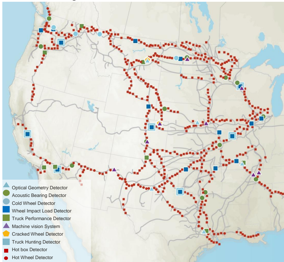
Figure 13: BNSF Track Detectors
